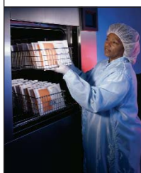
On the cover: Smith & Nephew's sterile processing operator loads medical implant devices into the VHP MD 2000 for the next sterilization cycle.
